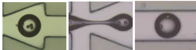
Figure 6: Keltone 1.75% capsules containing 30µm polystyrene beads.
