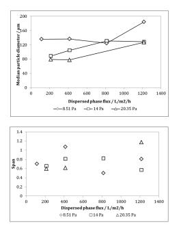
Figure 2. Effect of dispersed phase flux and shear stress on the median particle diameter
