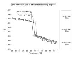
Figure 4. Phase transition temperature of different crosslinked pNIPAM hydrogels
