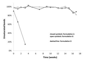
Figure 1 : Stability of encapsulated linseed oil in humid air (90% RH) at room temperature
