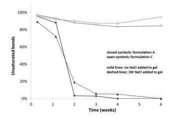
Figure 3 : Stability of encapsulated linseed oil in hydrogel matrix at 40°C
