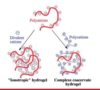
Figure 2. Schematic representation of two principles to form physical hydrogels.
