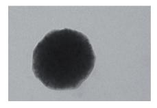
Figure 4: Transmission electron micrograph of layer-by-layer encapsulated magnetic emulsion. [4]
