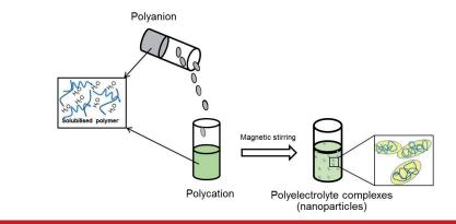
Figure 1. Schematic representation of the assembly of polyelectrolyte complexes.
