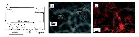
Fig. 3 Model for the magnetic delivery of polyelectrolyte capsules functionalized with magnetic nanoparticles (A). Living breast cancer cells attached to the bottom of the flow channel and located 11mm away (B) or just above the edge of the permanent magnet (C). Internalized capsules are recognized by their luminescence attributed to CdTe nanocrystals incorporated in the shells.
