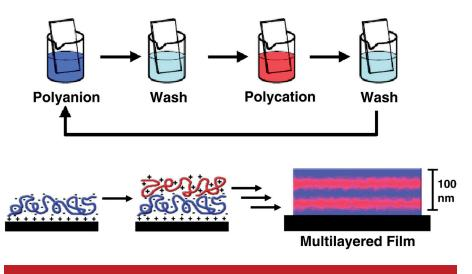
Fig. 2 A schematic representation of the alternate adsorption of the polyelectrolyte species to produce a multilayered structure
