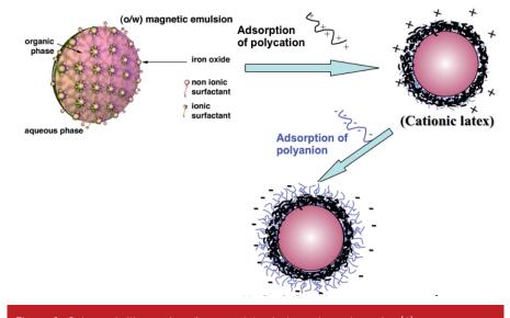
Figure 2 : Schematic illustration of sequential polyelectrolyte adsorption [4]
