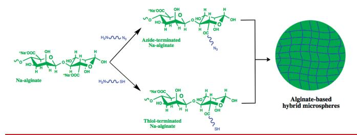
Figure 3. Functionalized Na-alg maintains the gelling capacity in presence of calcium ions and allows preparing chemical cross-linked networks.
