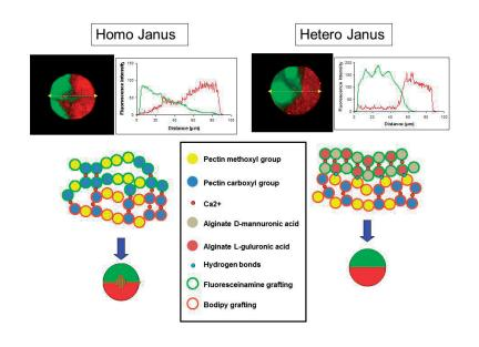
Figure 2. Fluorescence confocal microscopy images and profiles of the fluorescence intensities for FA-pectin/Bodipy-pectin homo Janus and FA-alginate/Bodipy-pectin hetero Janus microbeads. FA and Bodipy excitations were set at 488 and 561 nm, respectively, while emission fluorescence was recorded between 500 and 530 nm (green) and between 570 and 620 nm (red). Scale bars: 50 µm. The schematic explanations relative to the interface for both Janus microbeads are also given (see text for details).
