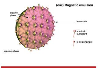
Figure 1 : Schematic illustration of oil in water magnetic emulsion
