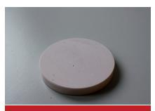
Figure 2. Fabricated sample composed of Ca-alginate microspheres incorporated into W19 commercially available low loss epoxy material.
