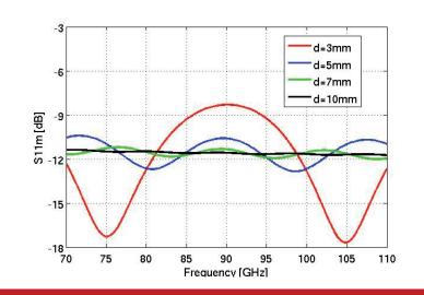
Figure 3. Simulated reflection coefficient of alginate composite material for different sample thicknesses.
