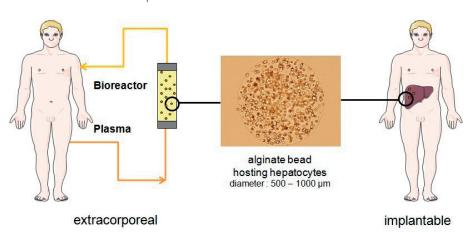
Fig. 1 : Concept of extracorporeal (EBAL) or implantable (IBAL) biortificial liver using hepatocytes encapsulated in alginate beads.
