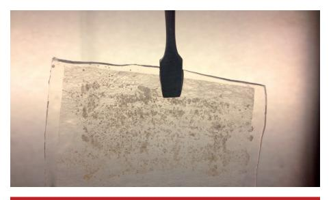
Fig. 1 Islet Sheet made from piglet islets, 3% alginate and polyester scrim
