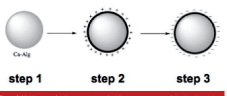
Figure 2: Multi-step technology, consisting of gel formatting, coating with polycation and polyanion, as well as washing steps, to adapt the physical properties for cell transplantation
