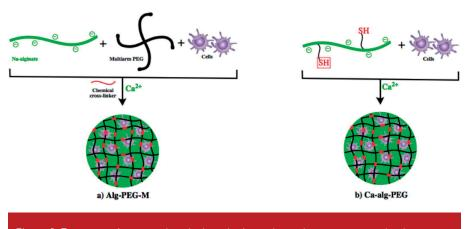
Figure 3: Two strategies to produce hydrogel microspheres by a one-step technology
