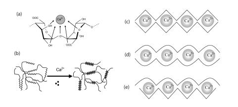
Figure 3. Crosslinking alginate polymers by calcium ions. Probably Ca-binding site in a GG-sequence (a) and ionic cross-linking of two homopolymeric blocks of G-residues by the egg-box model (b) [19]. (c) GG/GG junctions, (d) MG/MG junctions (e) GG/MG junctions [17].
