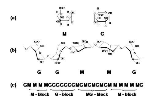
Figure 2. Structure of alginate. ß-D-mannuronic acid (M) and Đ-L-guluronic acid (G). Haworth formulas (a), ring conformation in the alginate chain (M: 4C1and G: 1C4) [6](b), and the alginate chain sequence (c).
