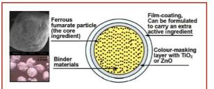
Figure 2. Schematic micro-particle structure and microscopic/SEM images of salt grain-size iron premix made by extrusion agglomeration and film-coating, with desirable characteristics suitable for salt and sugar fortification
