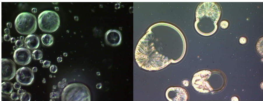
Figure 4: Vitamin A Palmitate containing microcapsules before (a) and after (b) glass slides compression (Average microcapsule size = 60 \mu\text{m} )
