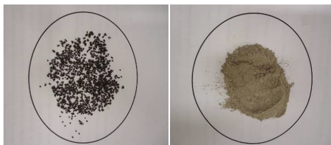
Figure 1. Lipase immobilized onto chitosan microparticles. A) Beads produced after cross-linking using sodium tripolyphosphate B) Powder produced after spray drying
