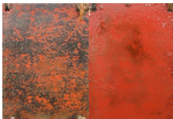
Figure 3. Ten month raft panel test results of copper-based: 45% Cu 2 O + 3% copper pyrithione (left), and copper-free coating: 5% Type 3 DCOIT microcapsule (right).
