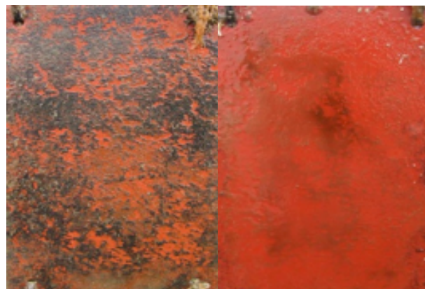
Figure 3. Ten month raft panel test results of copper-based: 45% \text{Cu}_2\text{O} + 3% copper pyrithione (left), and copper-free coating: 5% Type 3 DCOIT microcapsule (right).
