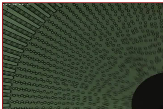
Figure 3: High-speed microscopic image of the exit of a multi-microchannel prototype device (EmulTech designed). Drops are 50 micron
