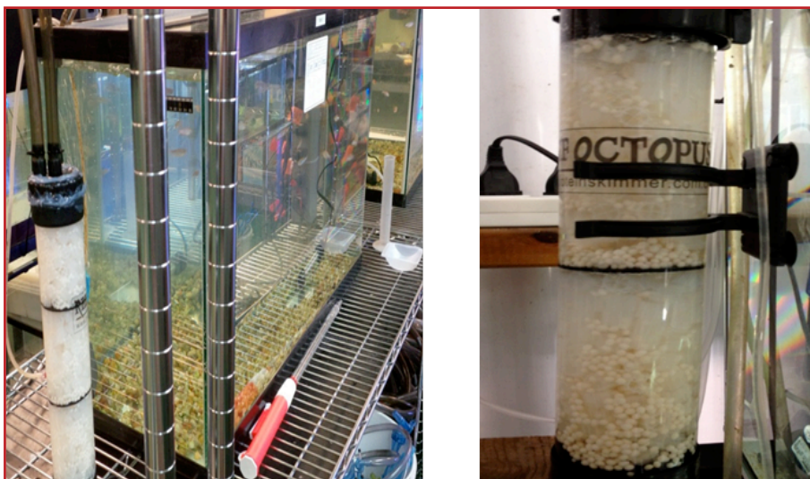
Figure 2. A prototype filter for nitrate removal in aquariums based on encapsulation of denitrifiers.
