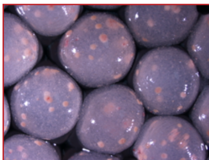
Figure 1. Immobilization of microbial inoculants in calcium–alginate beads by ionic gelation technique (beads 2–3 mm diameter).
